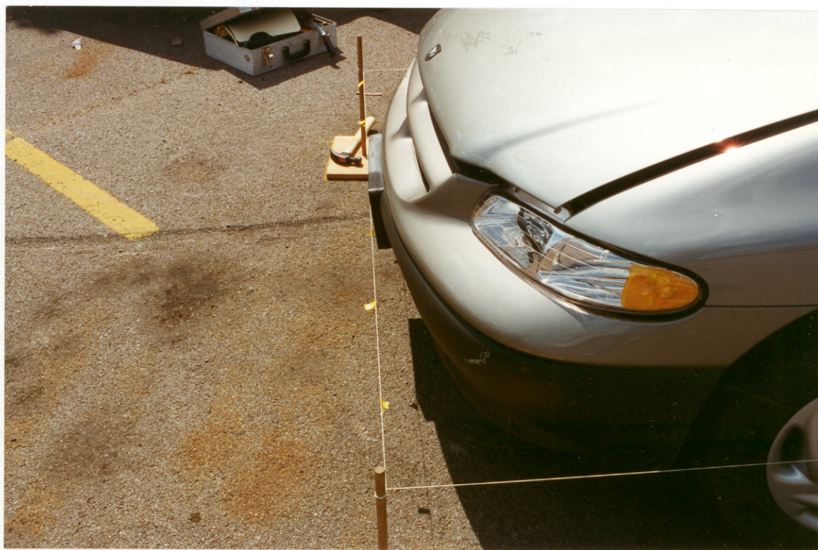
31. Left lateral view of the frontal crush to the Dodge Caravan.
